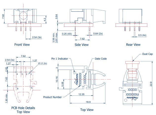
FIGURE 2 Mechanical dimensions of the horizontal connectors and PCB footprint, which is a top view General dimensional tolerance is  $\pm\,0.2~\text{mm}$
